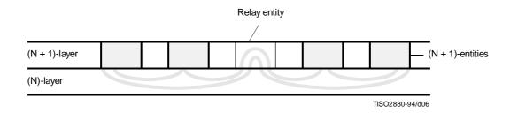
Figure 6 – Communication through a relay
