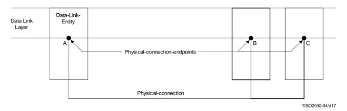
b) Example of a multi-endpoint-physical-connection (connection exists between A, B and C)
