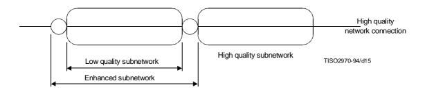
Figure 16 – Interconnection of an enhaned low quality subnetwork and a high quality subnetwork
