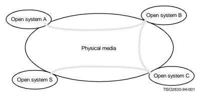
Figure 1 – Open systems connected by physical media
